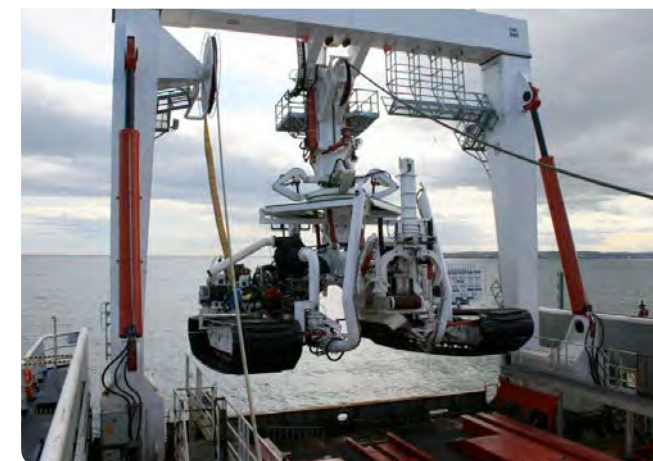
Figure 2-10 i-Trencher chain trenching vehicle & LARS
