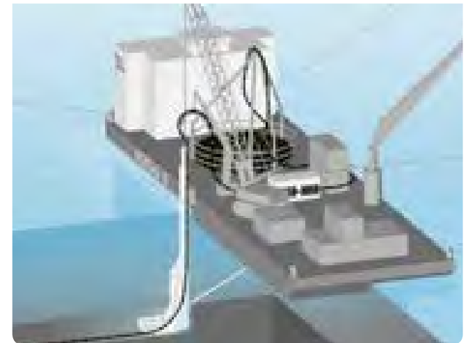
Figure 2-12 Schematic diagram showing the use of a jetting leg
